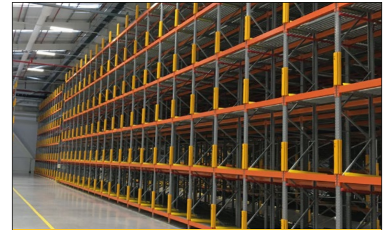
RackGuards can also be installed above ground level to protect racks from loading and unloading damage.
